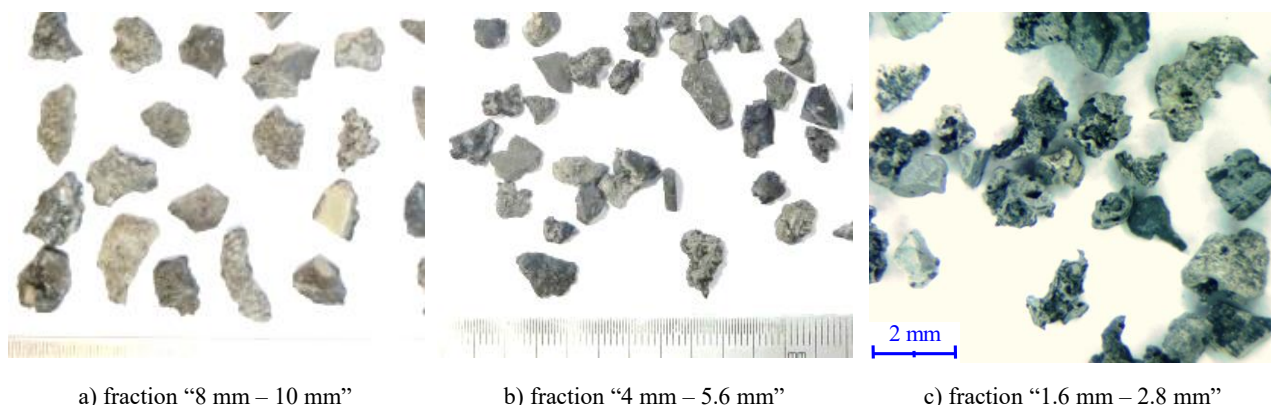
Figure 4. View of corium particles from the experimental container
