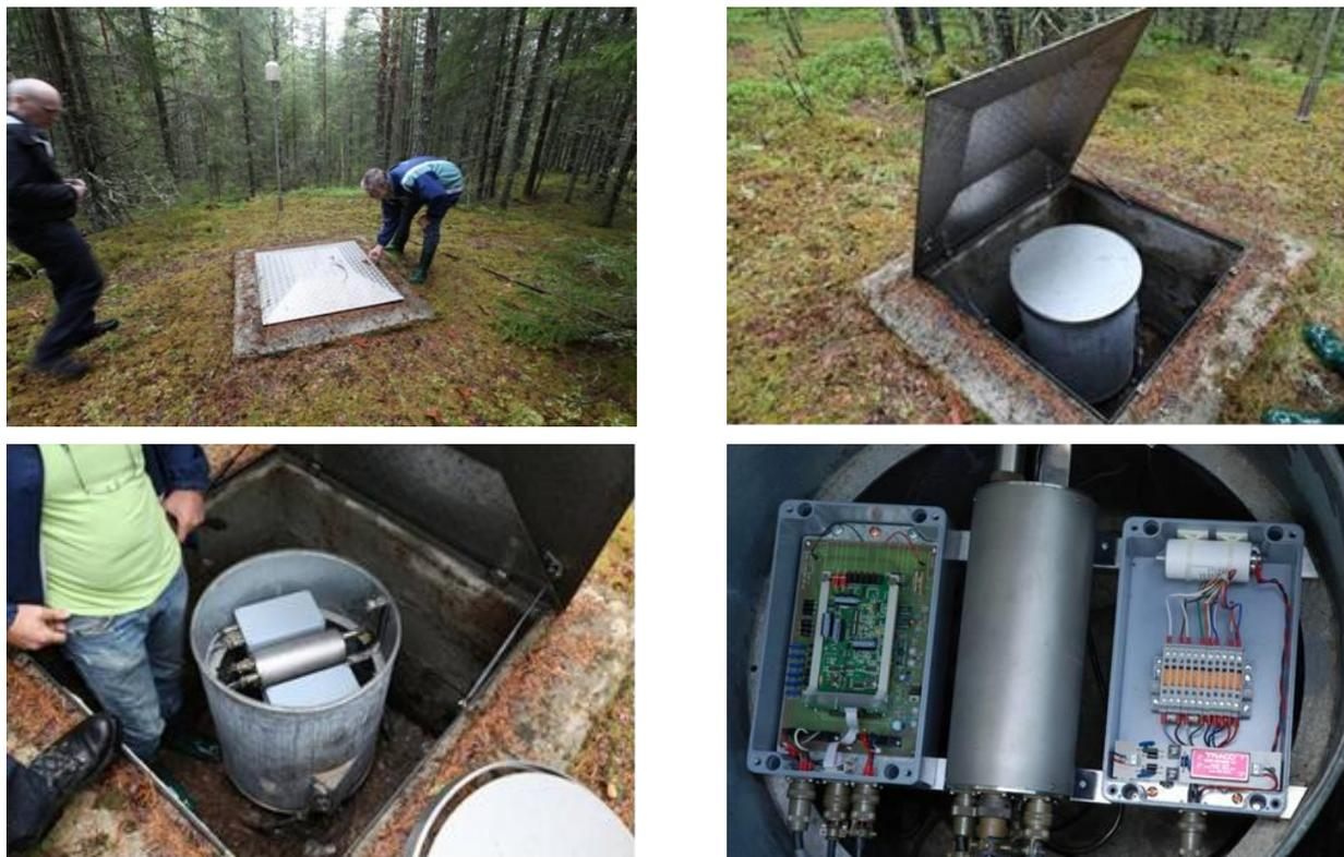
Figure 4. Borehole site (BS) NC601. The sensor is installed in a shallow (down to 12 m depth) borehole. A zinc drum on top of the borehole contains the digitizer (Güralp CMG-DM24S3EAM), a power and communication pit box (lightning protection, battery power charger, Patton modem, 12V 800mAh battery bank) and a junction box (coarse lightning protection and 48/12 DC/DC converter)
